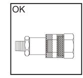
When making connections with quick couplers, make sure the couplings are fully engaged. Threaded connections such as fittings, gauges, etc. must be securely tightened and leak free. Never use excessive tightening force that may distort the fittings or strip the thread profile.
