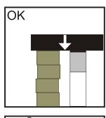
Place blocking or cribbing under the loads as you raise it. Each time you raise it higher, insert more blocking. Position yourself in a manner that will keep you clear of the load, and will not allow your hands or other body part between the load and the cribbing.
