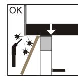
Weld splatter will damage plunger rods and hose. Hydraulic fluid can ignite if vaporized or exposed to high temperatures.
