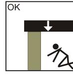
As with jacks, never place any part of your body under the load. Load must be on cribbing before venturing under.
