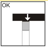
Don't use cylinder without saddle. This will cause plunger to "mushroom". Saddle distribute load evenly on the plunger.
